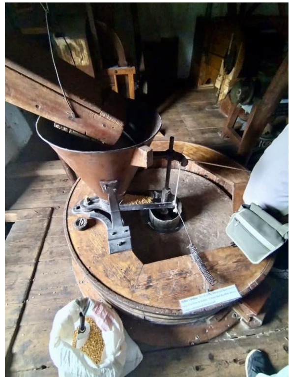
Figure 5: Inside the Mill, grain poured down the chute falls under the millstone, producing various sizes of ground grain. (Photo: Britney Hawkins)
